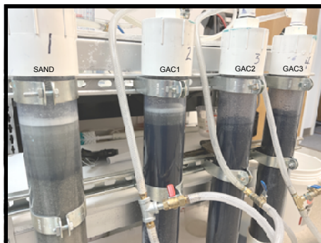
Figure 5: PFAS Foam Removed by 1st GAC Column
