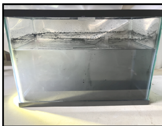
Figure 8: Post 48-Hour Clarification after 1,000 mg/l PAC Treatment
