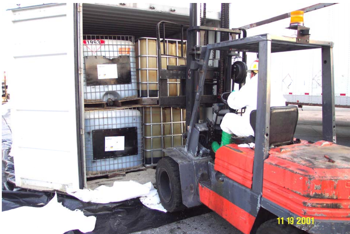
CASE 1-2: Leaking intermediate bulk container on top right.
