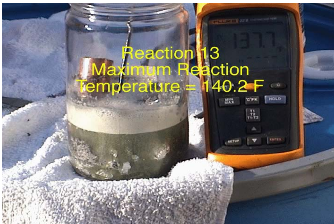
CASE 3-4: Heat of reaction test yields maximum temperature of 140.2 F - considerably below autoignition temperature for paper or cloth.
