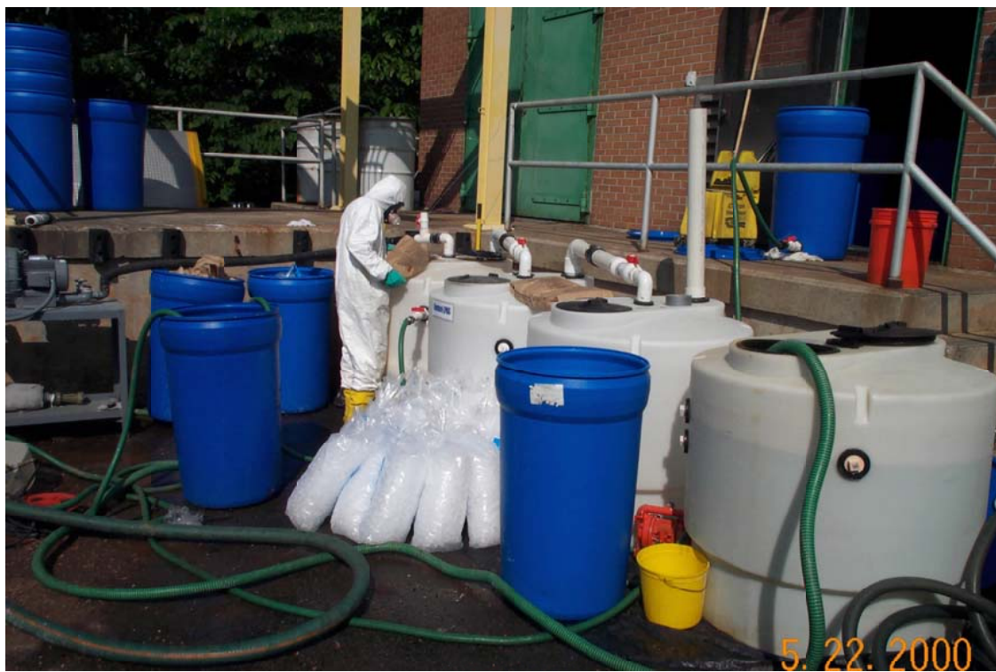
CASE 2-4: Addition of reactants and Ice to reactors stabilize sodium chlorite and control the heat of reaction.
