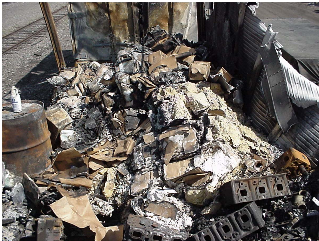
CASE 3-2: Chemical burn residues in middle trailer where fire started.
