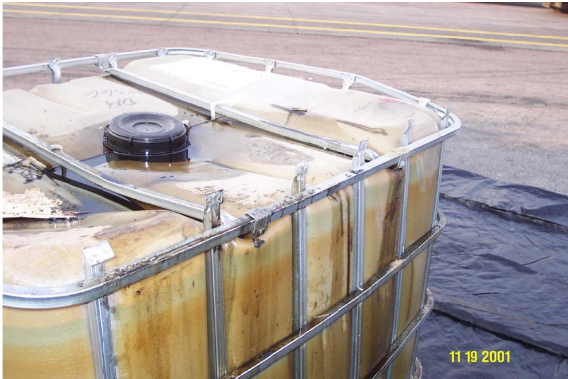
CASE 1-3: Failed top ring connectors allowed vertical supports to puncture second layer container.
