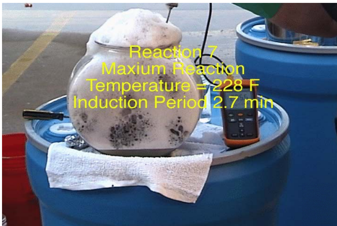
CASE 3-3: Heat of reaction test with 10% sodium hydroxide and metal catalysts (aluminum, steel wool, copper, and brass).
