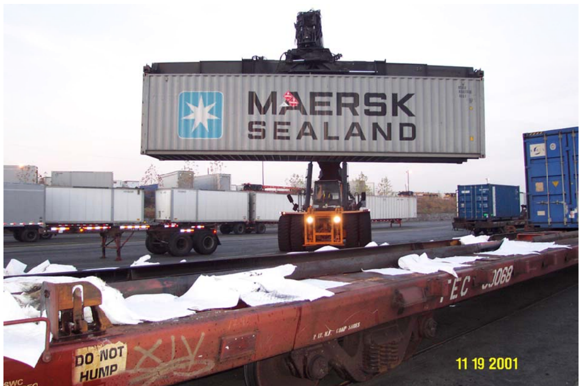
CASE 1-1: Leaking intermodal container removed from rail flatcar for integrated remediation and root cause determination.
