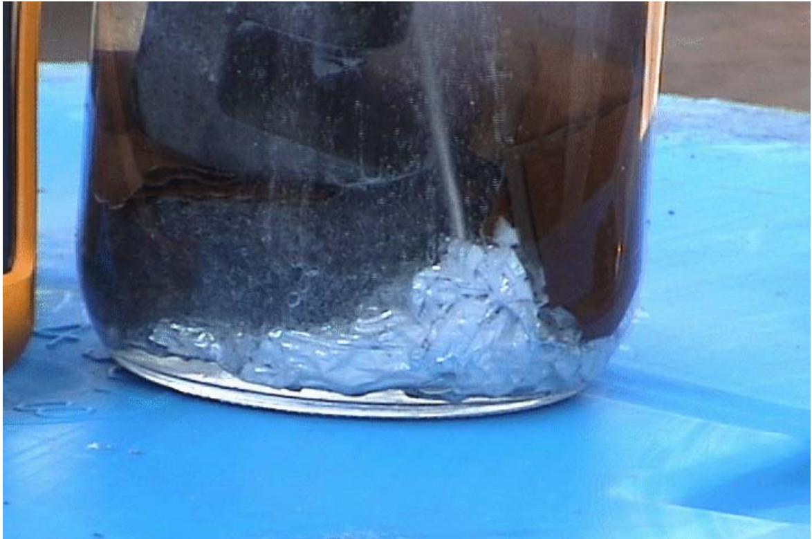
CASE 3-6: Close up of heat of reaction test with 10 - 30% phosphoric acid and metal catalysts (copper, brass, aluminum, steel wool)
