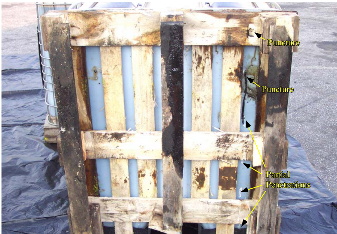
CASE 1-4: Bottom of second layer tote punctured by vertical supports of first layer tote.
