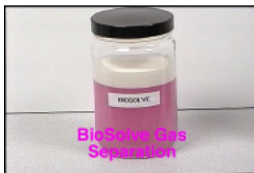
Photo 15: Gasoline Separates from BioSolve Emulsion
