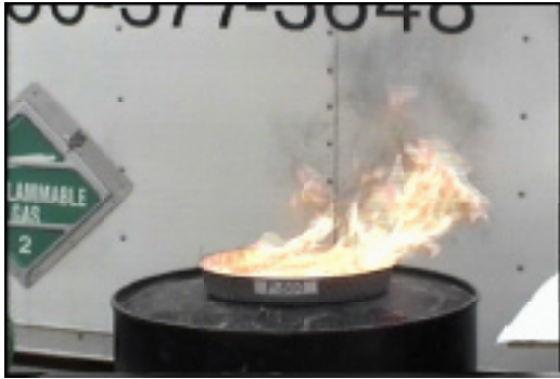
Photo 1: F-500 1:8:32 (product:gasoline:water) ratio ignites
