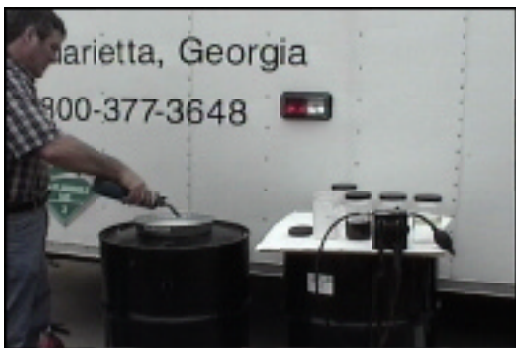
Photo 4: Alcoseal 3-6 Does Not Burn at 1:8:32 ratio.
