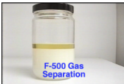
Photo 14: Gasoline Separates from F-500 Emulsion
