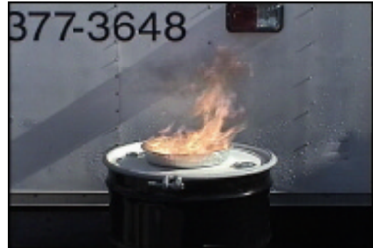
Photo 7: BioSolve ignites at 1:6:33 ratio (3%)
