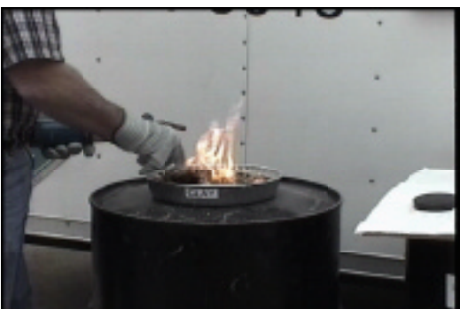
Photo 12: Stirring Clay Blanket Allows Gasoline to Ignite
