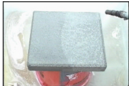
Photo 22: F-500 Cleaning - Left Side of Block - Diesel, Right Side - Hydraulic Oil. Note Water Beading Up on Block Face Indicating Oil Film Remaining
