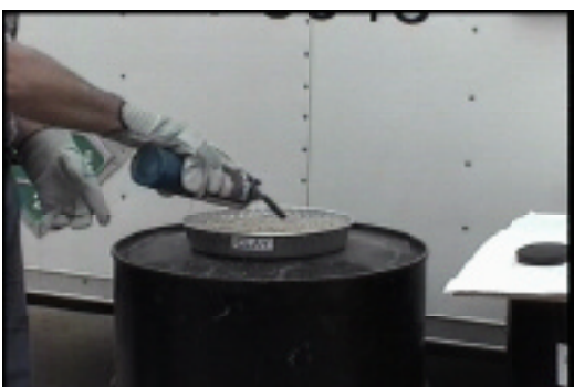
Photo 11: Oil Dry Blanket Prevents Gasoline/Water Ignition
