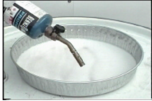
Photo 5: HC-2000VAP does not burn at 1:8:32 ratio (3%)
