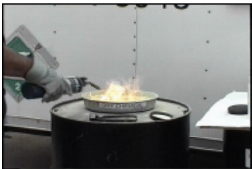
Photo 10: Dry Chemical Media Ignites on Stirring
