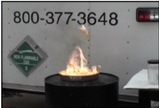
Photo 2: F-500 2:8:32 (product:gasoline:water) ratio ignites
