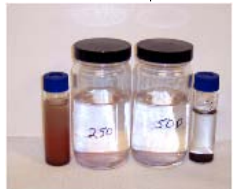
PAC & Calcium Chloride Dye Treatment
